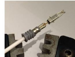
4. Proper crimp. Make sure the terminal retains the seal as shown.
