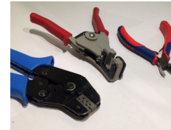
1. Typical termination equipment
