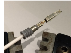
4: Proper crimp. Make sure the terminal retains the seal as shown.
