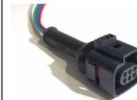
7. Finish the termination job by fixing the grommet into place.
