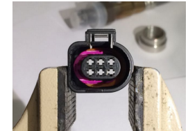
6: After all terminals are inserted and locked, push the pink secondary lock into place from the left side.
